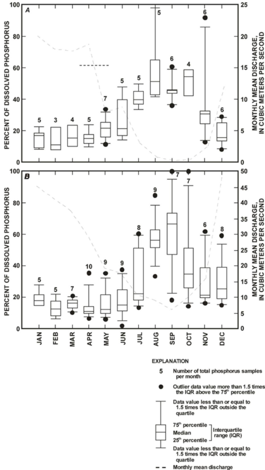
Figure 7. Percentage of dissolved phosphorus in the stream compared to monthly mean discharge from point samples taken at (A) the Tensas River at Tendam, LA, 1995 to 2000, and (B) the Bogue Phalia near Leland, MS, 1996 to 2001.
