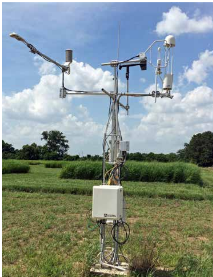
Figure 2. Eddy covariance system in Stoneville, MS for long-term agroecosystem monitoring and assessment.
