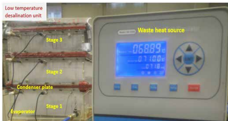
Figure 2. Low temperature desalination unit powered by waste heat source, photo image of the experimental setup.
