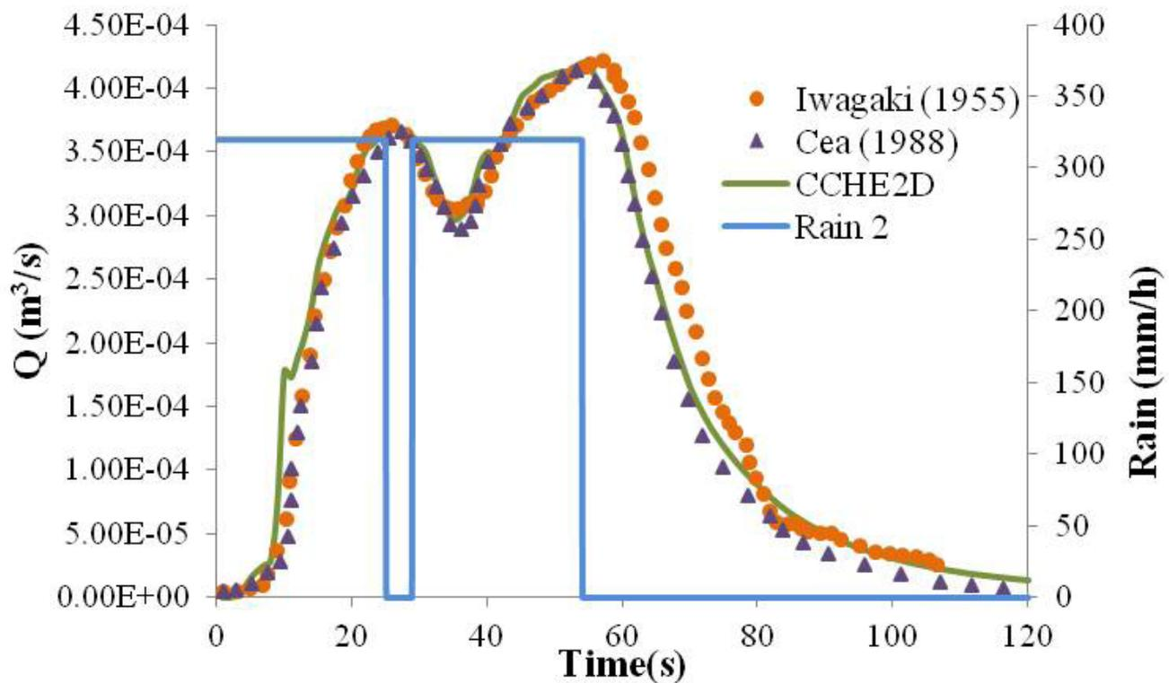
Figure 7: Runoff hydrograph for 2D validation test case 2C
