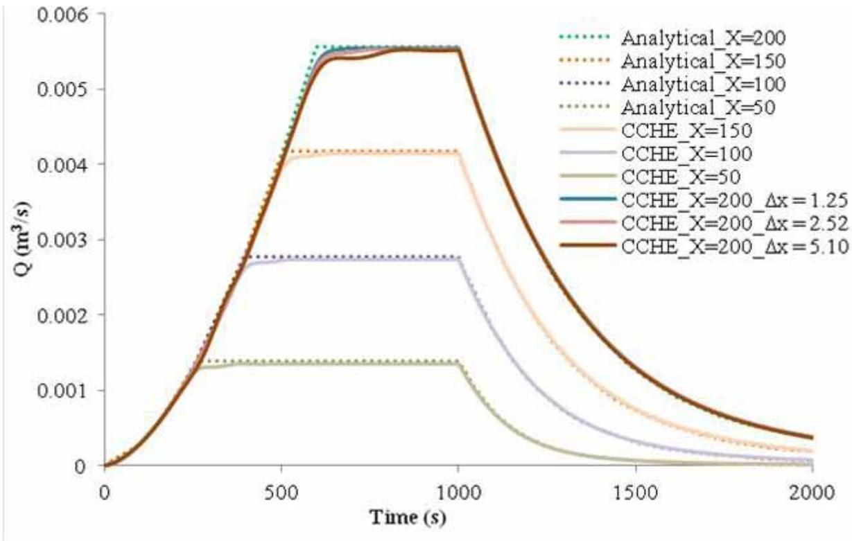
**Figure 2: Runoff hydrograph for analytical solution and numerical solution by CCHE 2D for rainfall of finite duration.**
