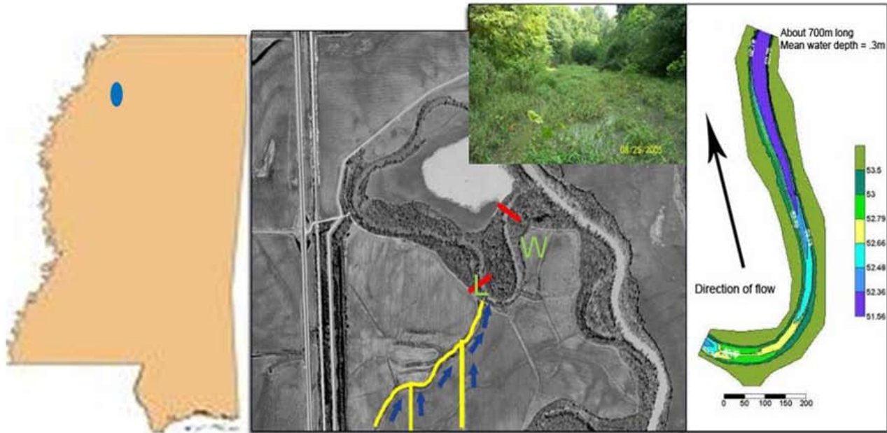
Figure 1. Managed wetland on west side of Coldwater River, Tate and Tunica Counties, MS. Inset photo shows wetland prior to construction of weirs used to manage water levels, which are shown as red bars on aerial photo. Blue arrows along drainage ditch and slough (shown in yellow) indicate the flow in the channels of runoff from about 100 ha of cultivated lands. Wetland topography shown on contour map to right; elevations are in m referenced to NAVD 88. Site location shown on map to left.
