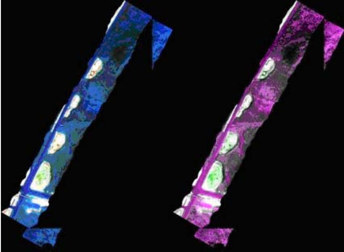
Figure 2. The original (left) and the corrected (right) subset image of airborne AISA data obtained over seagrass beds in Mission-Aransas National Estuarine Research Reserve, TX.
