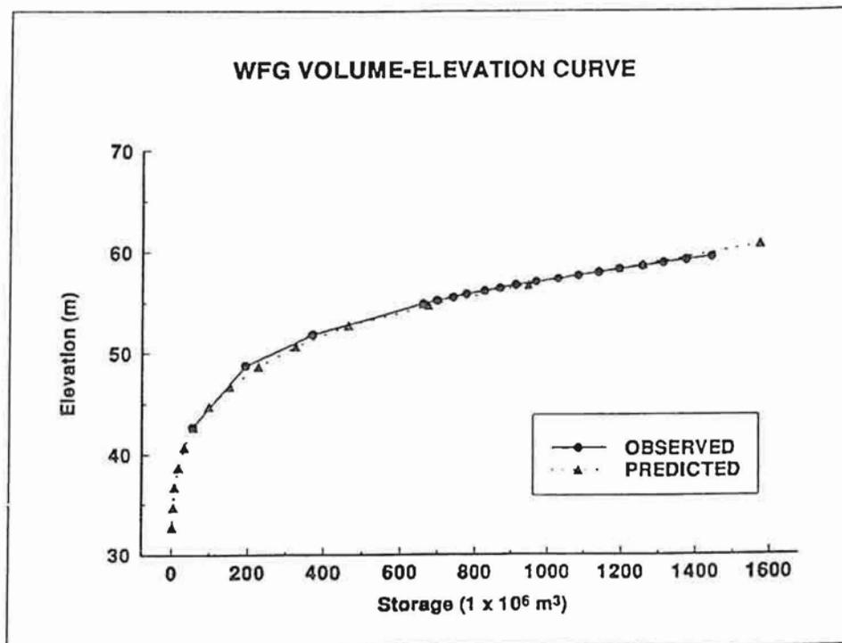
Figure 3. Walter F. George Reservoir computed versus observed volume elevation curves
