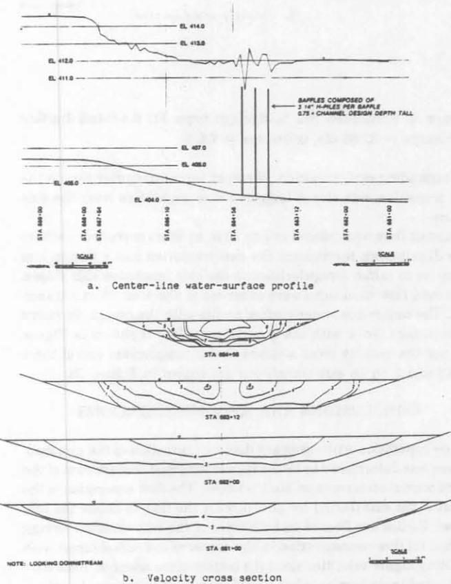
Figure 3. Structure No. 5, design: type 3C, 6.2-ft-tall baffles, discharge = 2,355cfs, tailwater = 8.2 ft.
