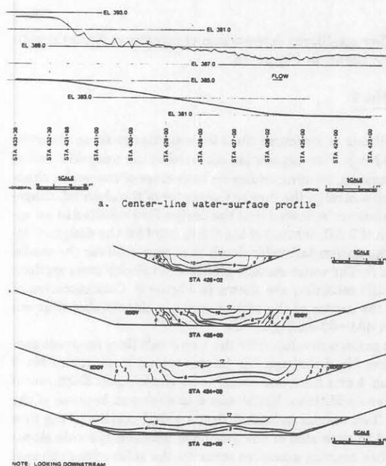
Figure 5. Structure No. 2, original design, discharge = 3,166 cfs tailwater = 7.6 ft.
