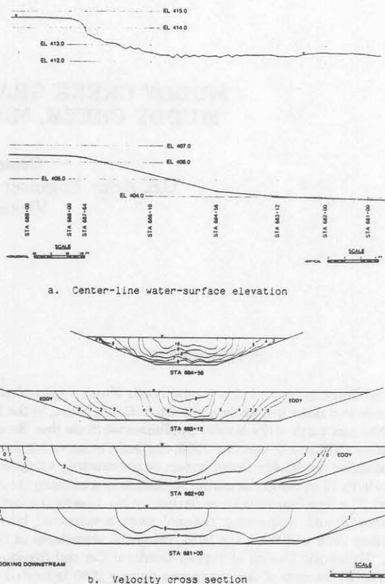
**Figure 2. Structure No. 5, original design, discharge = 2,335 cfs, tailwater = 8.5 ft**
