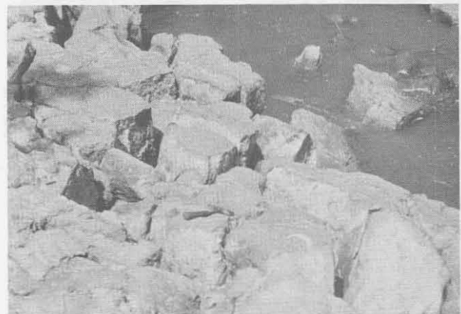
Fig. 14. Close-up of Old Paleosol Block Failure
