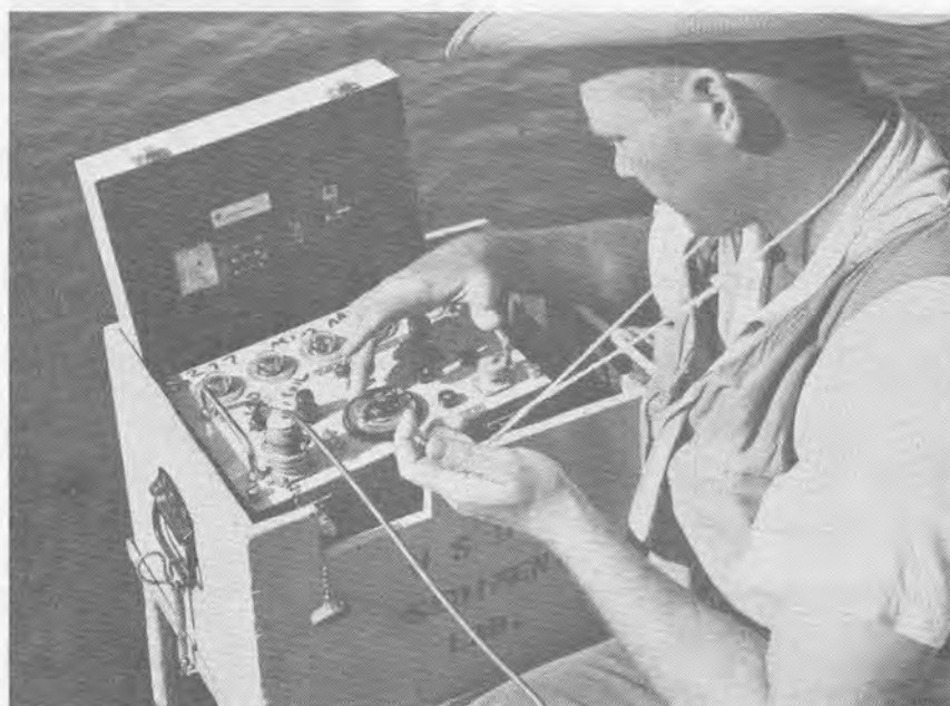
Figure 5. Operator taking a measurement. The radiation intensity "seen" by the GM tubes in the gamma probe is read out by this scaler. A stop watch is used to time the measurement period. Note the cable connecting the scaler to the probe.
