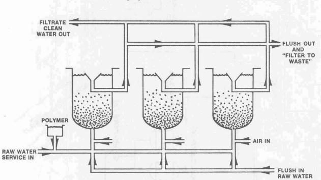
FLOW DIAGRAM utilizing open or closed vessels
