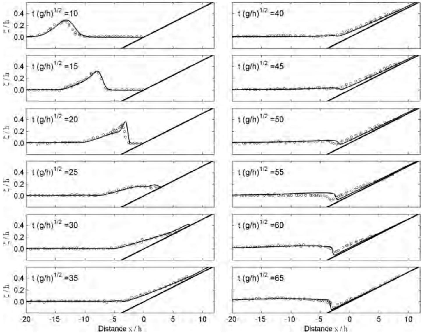
**Figure 6. Surface profiles of a solitary wave propagation over a fringing reef. Numerical results (solid lines), experimental data (circles).**
