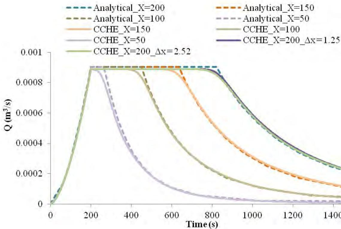
Figure 3: Runoff hydrograph for analytical solution, experimental data (Gottardi et al. 2008) and numerical solution by CCHE2D
