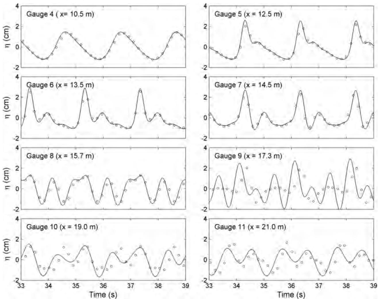
**Figure 5.** Surface profiles of a solitary wave run-up on a 1:19:85 plane beach. Numerical results (solid lines), experimental data (circles).
