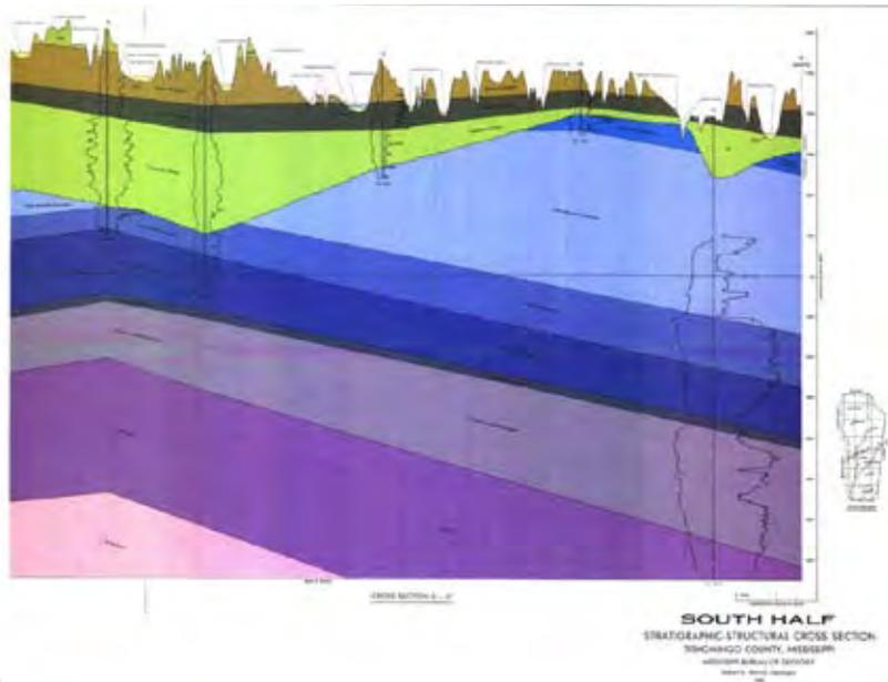
Figure 1. South half of a north-south cross section through Tishomingo County, Mississippi, by Bob Merrill (1988), showing the thickening of the Tuscaloosa Formation (green) within a valley cut into the Paleozoic bedrock.
