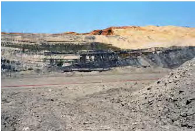
Figure 9. Lignite seams bend beneath a fluvial channel sand (upper right) in the middle Tuscahoma Formation, which cuts out the I and H2 lignite seams. The red cable carries 60,000 volts to power the dragline. Picture (color negative 531-16) taken on November 11, 2004.
