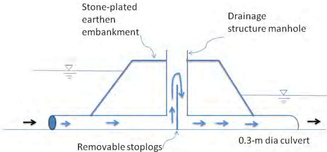
Figure 2. Schematic of drainage structures and weirs shown as red bars in Figure 1.
