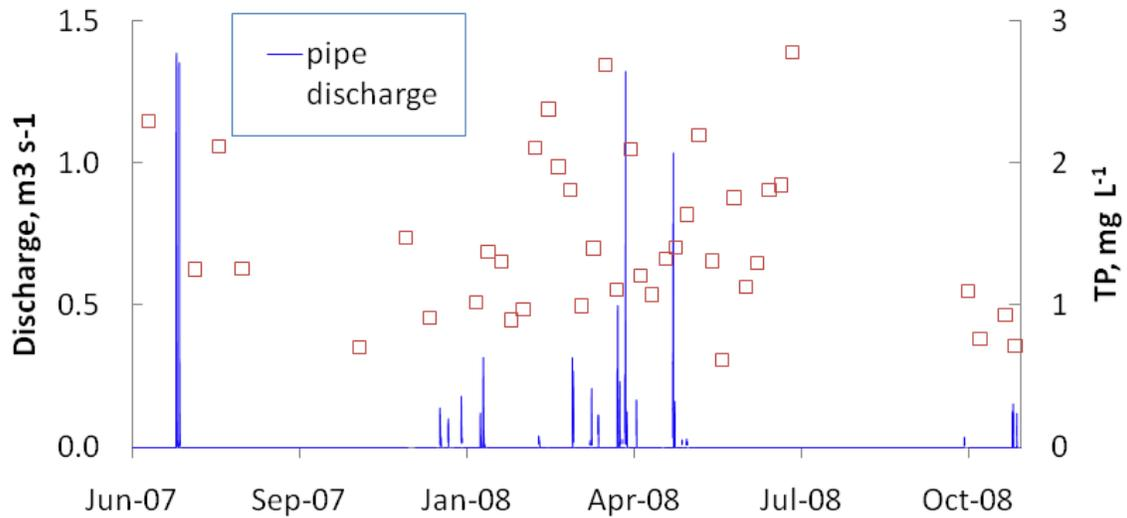
Figure 5. Discharge through tributary pipe versus date and total phosphorus concentration in tributary slough during study period.
