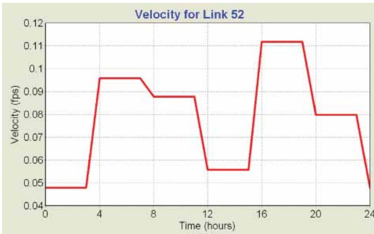
**Figure 8.** Velocity Variation for Water Supply Point with Highest Velocity (Link 52)
