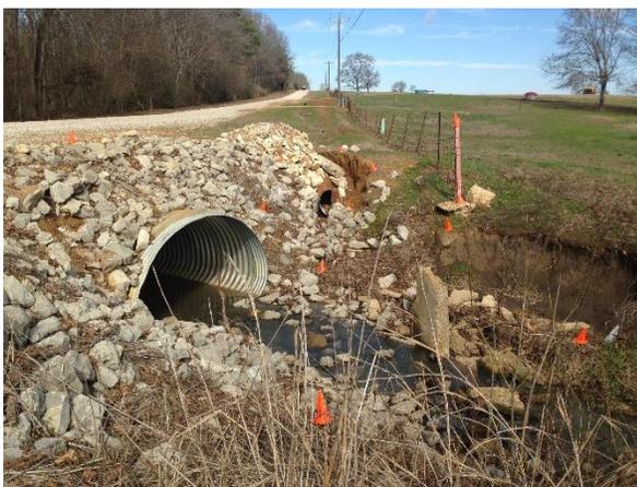
*Preliminary trials on structure for motion using soccer cones for reference points. We measure between the cones on the ground and in the image to validate our 3D surface model.*
